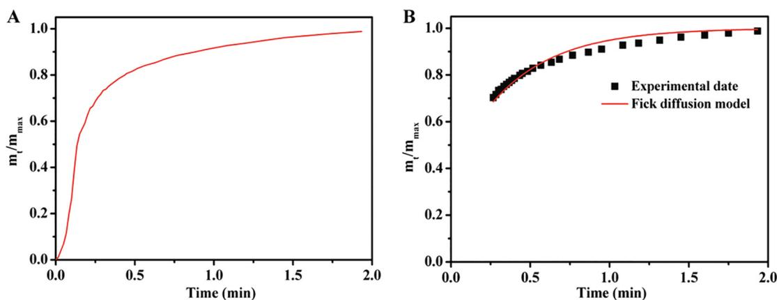
Fig. 7. (A) Adsorption kinetic of  $\text{SO}_2$  at 298 K for HNIP-TBMB-1 and (B) Fick's diffusion model on experimental  $\text{SO}_2$  uptake of HNIP-TBMB-1.
