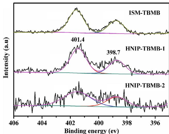
Fig. 4. XPS N 1s spectra of ISM-TBMB and HNIP-TBMB.
