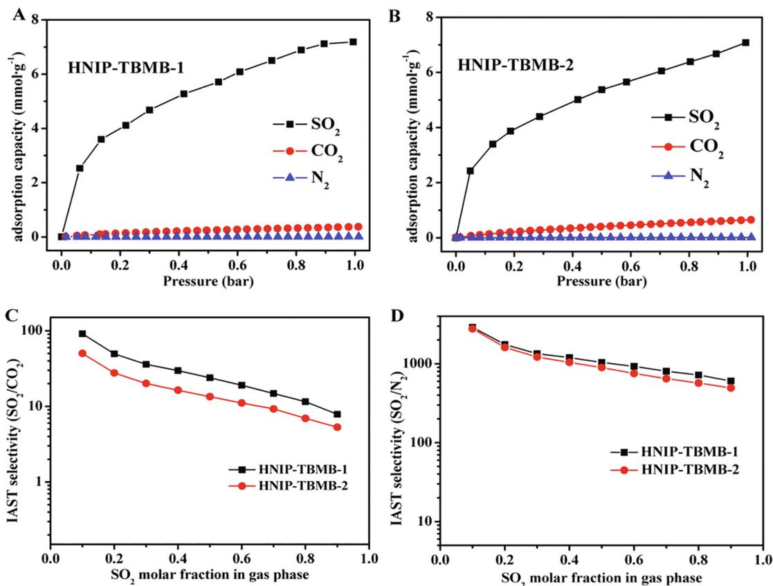
Fig. 5. SO<sub>2</sub>, CO<sub>2</sub>, and N<sub>2</sub> adsorption isotherms for A) HNIP-TBMB-1 and B) HNIP-TBMB-2 at 298 K and 1 bar. The IAST selectivity of C) SO<sub>2</sub>/CO<sub>2</sub> and D) SO<sub>2</sub>/N<sub>2</sub> mixtures with varying SO<sub>2</sub> molar fractions in gas phase at 1 bar.
