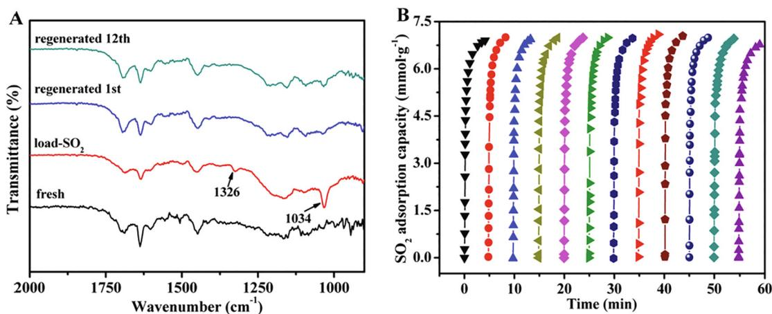
Fig. 9. A) FTIR spectra of fresh,  $\text{SO}_2$ -loaded, 1st regenerated, and 12th regenerated HNIP-TBMB-1. B) Recycle performance of HNIP-TBMB-1 for  $\text{SO}_2$  adsorption.
