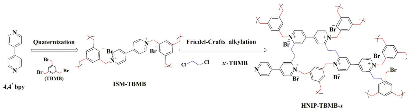
Scheme 1. The two-step synthesis procedure of HNIP-TBMB-*x*.
