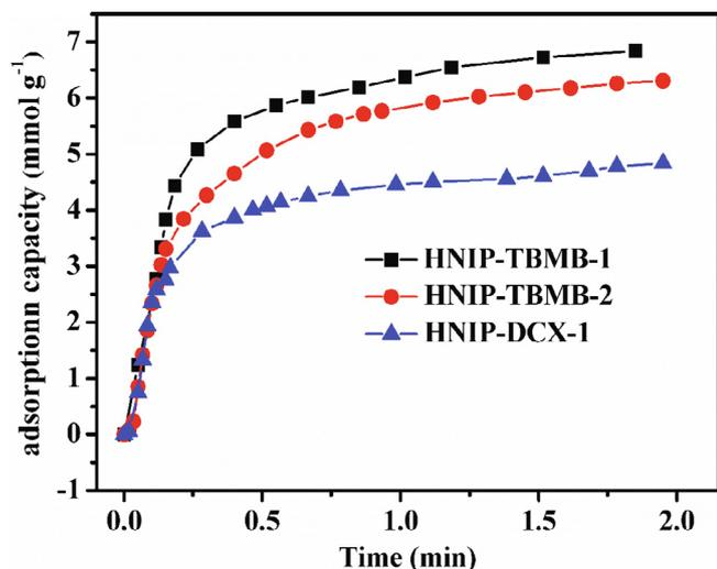
Fig. 6. SO<sub>2</sub> adsorption rate for HNIP-TBMB and HNIP-DCX at 298 K and 1 bar.
