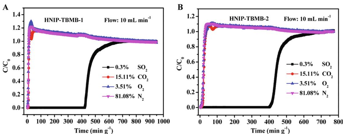
Fig. 8. Experimental column breakthrough curves of A) HNIP-TBMB-1 and B) HNIP-TBMB-2 for simulated flue gas compositions.
