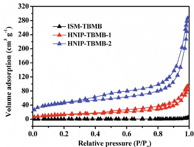
Fig. 3. N<sub>2</sub> adsorption/desorption isotherms of ISM-TBMB and HNIP-TBMB.
